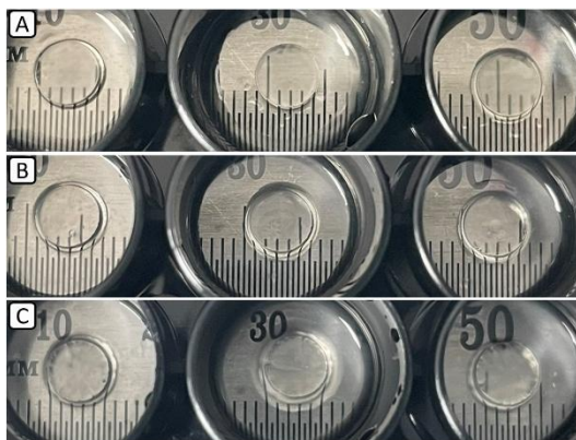
Figure 2. Representative images of PEGDA-INK constructs (5 mm diameter, 1 mm height) using layer-by-layer mode with 1 layer of 1 mm exposed for 3.5 s with 75% intensity (A), 10 layers of 100 \mu m exposed for 1 s per layer with 100% intensity (B) and continuous mode with 0.06 mm/s (C), after overnight PBS incubation.
