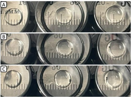
Figure 2. Representative images of constructs (5 mm diameter, 1 mm height) printed using layer-by-layer mode with 1 layer of 1 mm exposed for 30 s with 80% intensity (A), 10 * 100 μm layers with 5s/L at 100% (B) and continuous mode with 0.025 mm/s at 100% (C) after overnight PBS incubation.
