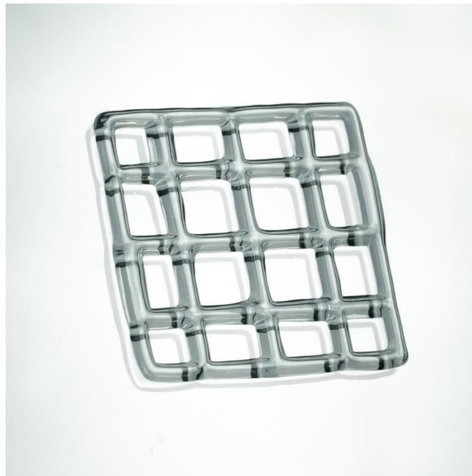
Figure 2. Three-layered grid structure, 20 x 20 mm, acquired after printing with the parameters in Table 2 with CELLINK START.
