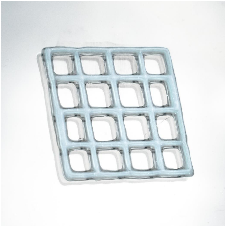
Figure 2. Three-layered grid structure, 20 x 20 mm, acquired after printing with the parameters in Table 2 with CELLINK RGD mixed with PBS (10:1). The picture was taken prior to ionic crosslinking.
