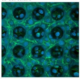
3D printing of microwell arrays for cell cultivation printed using IP-S.
