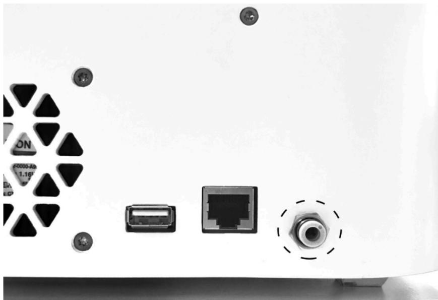
**Figure 6:** External air supply inlet. A 4-mm air tube can be inserted into the BIO X using the pneumatic connector located on the back of the device.
