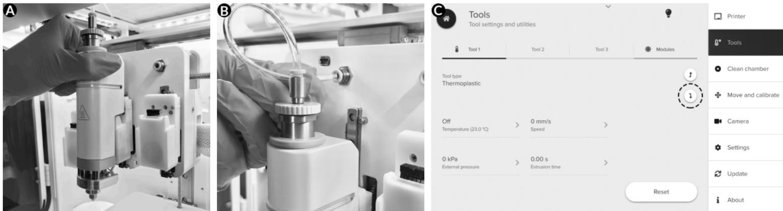
**Figure 9:** (A) Attaching the Thermoplastic Printhead to the mount. (B) Attaching the airline to the printbox. (C) Lowering the printhead to the active position.
