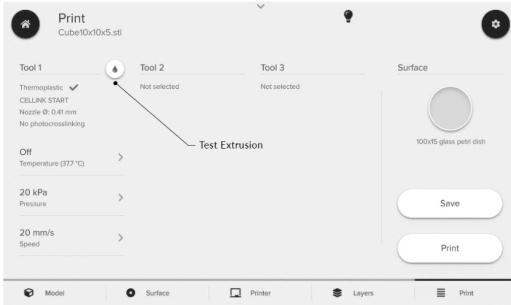
**Figure 16:** Print menu. You can preview your printing parameters and test the pressure. You can also adjust parameters on this menu. Press Print to proceed to the calibration page and press Save to save the configuration as a protocol.
