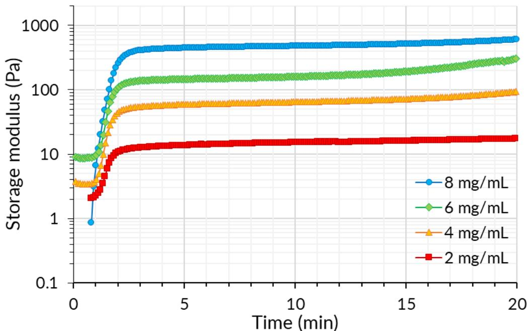
**Figure 1.** Thermal gelation of neutralized Coll 1 solution with different collagen concentrations ( $C_F$ ) indicated as storage moduli increase over time at 37°C.
