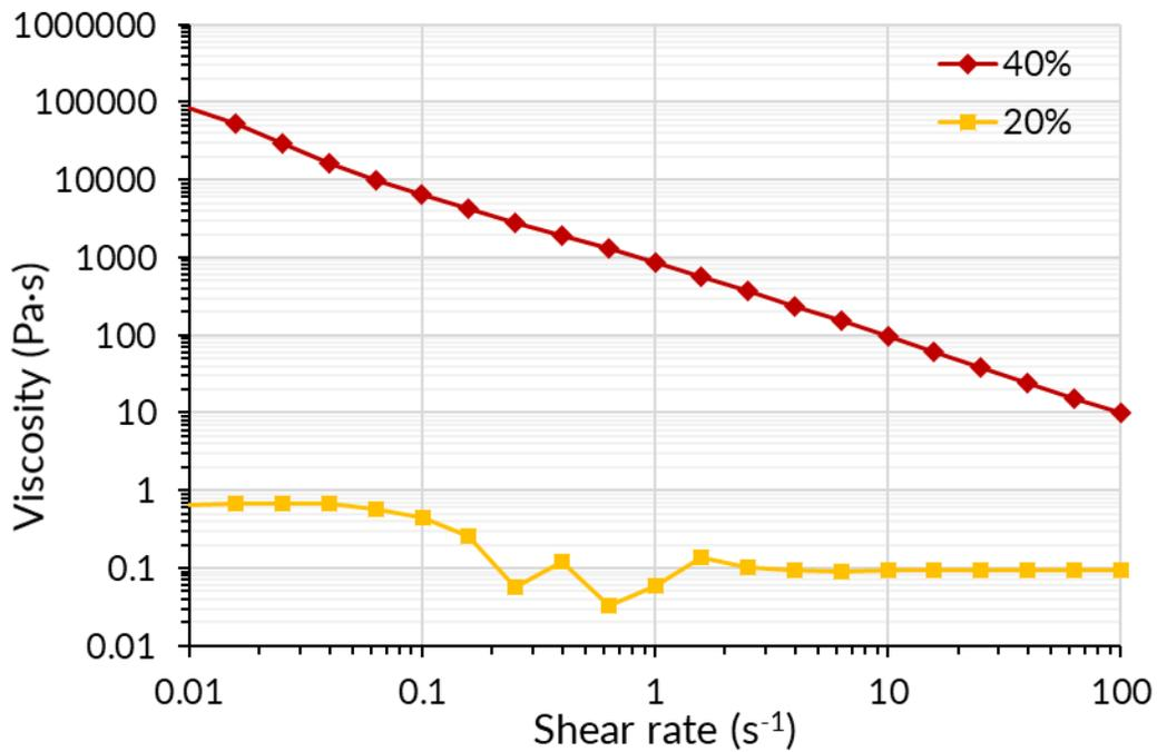
**Figure 1.** Viscosity of Pluronics dissolved in deionized water at 20% and 40% over a shear rate range of 0.01 to 100 s<sup>-1</sup>, 25°C.
