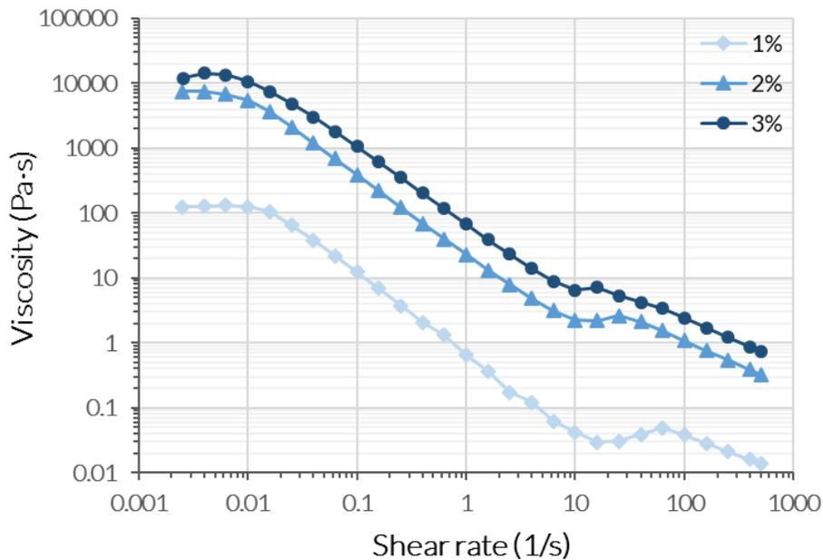
**Figure 1.** Viscosity of CELLINK Nanofibrillated Cellulose diluted with Reconstitution Agent M (sugar solution, available at CELLINK web store) to different concentrations over a shear rate range of 0.002 to 500 s<sup>-1</sup>, 25°C.
