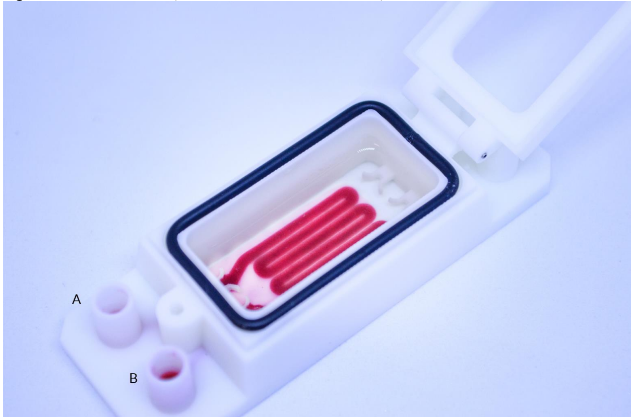
Figure 1. Show A, luer slip connector out and B luer slip connector in.
